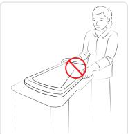
Remove CloudCover. Do not remove GelMat during cleaning.
