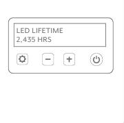
System will display LED lifetime\*\*. Verify that time is less than 25,000 hrs.
