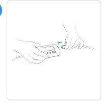
Attach Controller and Power Supply to device and place Controller outside enclosing walls of treatment area.
