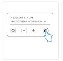
Press and hold power button to START device. System notifies once self-check completed\*.
